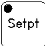
This LED indicates that the CarbPC is in the data entry mode for the setpoint and alarm parameters.
