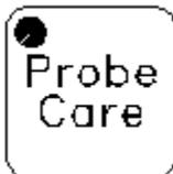
This LED indicates that the CarbPC is in the data entry mode for the probe care parameters. This LED also indicates by flashing that a probe care cycle is in progress or a Probe Care alarm condition exists.
