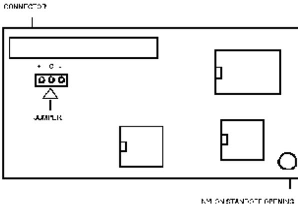
The thermocouple jumper selects either a full upscale or a full down scale reaction to take place when a thermocouple fails or becomes open. The jumper can be found on the thermocouple board, and has two possible settings (see Figure). For full scale upwards, place the jumper from the + to the C, and for full scale downwards, place the jumper from the - to the C.
