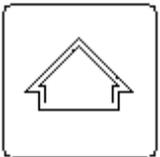
This key is usually used to increase the value of a digit in the data entry mode or scroll through various parameter sequences. In Manual mode this key will cause the control action to move in the Output 1 direction. When used in the dual-key operation Shift/"up arrow" an LED test is activated, where every segment and decimal point should light in both displays. If any segment or decimal point does not light a keyboard problem may exist, contact a qualified MSI representative.
