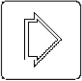
This key is usually used to select which digit is to be modified in a data entry mode. In Manual mode this key will cause the control output to go to the full Output 1 direction. In the Programmer Status Display mode it causes the display to move to a new page.
