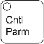
This key selects the Control Parameter Enter mode where the Proportional Band, Reset, Rate, Cycle Time and Percent Output values (if in solenoid mode) can be accessed and altered. When used in the dual-key operation Shift/Cntrl Parm it selects the keyboard Lock Level change mode.
