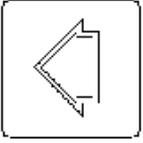
This key is usually used to select which digit is to be modified in a data entry mode. In Manual mode this key will cause the control output to go to the full reverse control direction while the value is displayed in the SET window. In Automatic mode pressing "left arrow" causes the % on-time valve position to be displayed in the SET window. (positive-Output 1, negative-Output 2). In the Programmer Status Display it causes the display to move to a new page.\*\*
